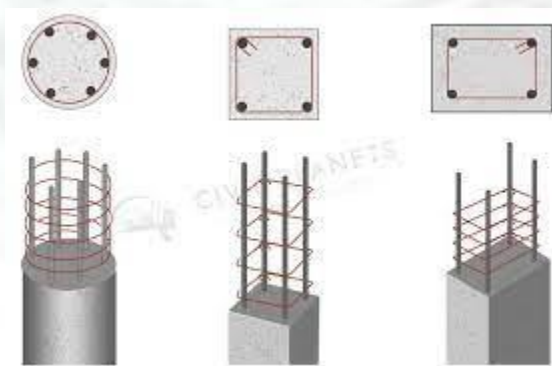
Different shape of the column with reinforcement
