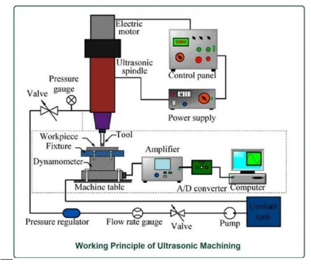
Ultrasonic Machining is process in which the Harder material is machined. These machines have great properties like
