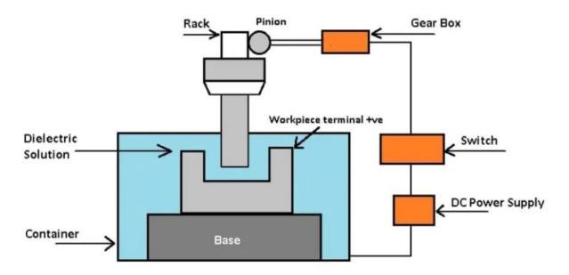
**Electric discharge machining,** also known as spark erosion, electro-erosion or spark machining, is a process of metal removal based on the principle of erosion of metals by an interrupted electric spark discharge between the electrode tool cathode and the working anode.
