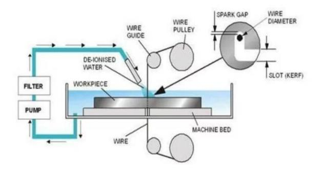
Wire electrical discharge machining is a non-contact subtractive manufacturing process that uses an electrically charged thin wire with a dielectric fluid to cut a metal part into different shapes.
