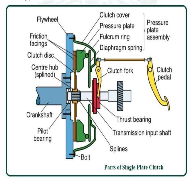
The flywheel is attached on the engine crankshaft and rotates with it. A pressure plate is bolted to flywheel through clutch spring, which provides the axial force to keep the clutch engaged position, and is free to slide on the clutch shaft when the clutch pedal is operated.
