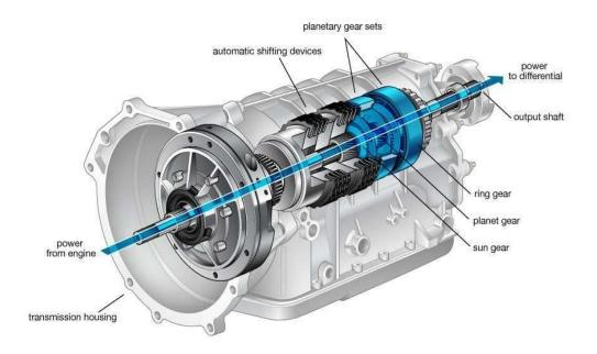
The gear shifting from one gear to another gear is done through hydraulically operated pistons by actuating springs. These springs control the brake bands on the planetary gear sets and clutches within the planetary unit. The various shifts achieved by the throttle and centrifugal governor.
