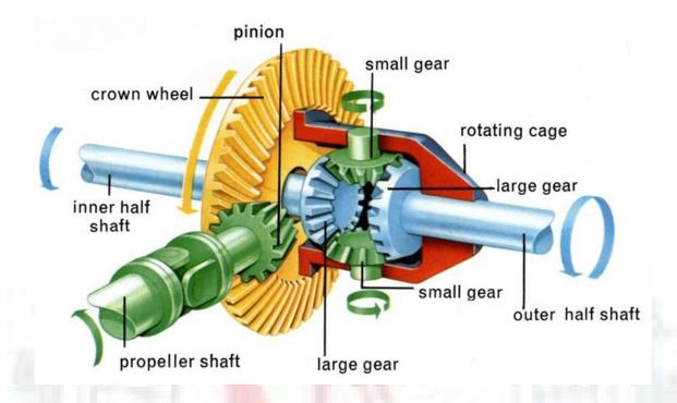
The differential is a very important part in a vehicle, as a component transfer, the engine power is transmitted to the wheels. Engine power is transferred by a rear propeller shaft to the wheel first changed direction by differential rotation are then referred to rear axle shafts after that to the rear wheels.
