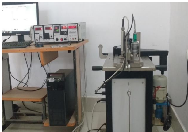
Fig. 2.8. Pin on disc set-up
