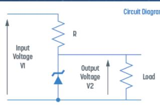
**Anode:** The anode is typically connected to ground. If a positive voltage is applied to the anode, it will conduct like a regular diode.
