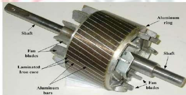
(b) Squirrel cage rotor
